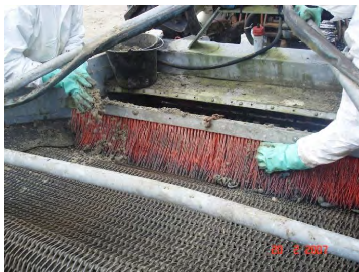
Mechanical sand/gravel/pebble sieving (Source: Le Floch Depollution)
